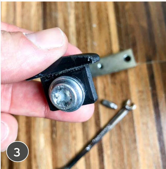
3 The hole cover is attached with the same original Torx screw.
