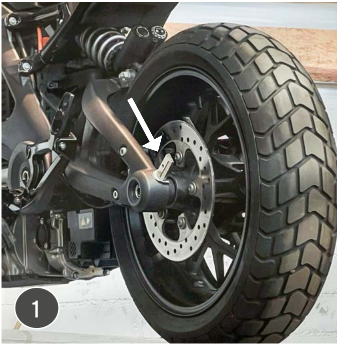
1 After removing the rear bow, a bracket remains on the left swing arm.
