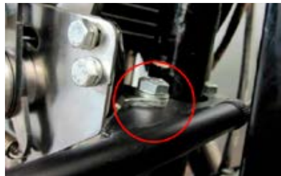
Placement of rear shifter ratchet support angle
