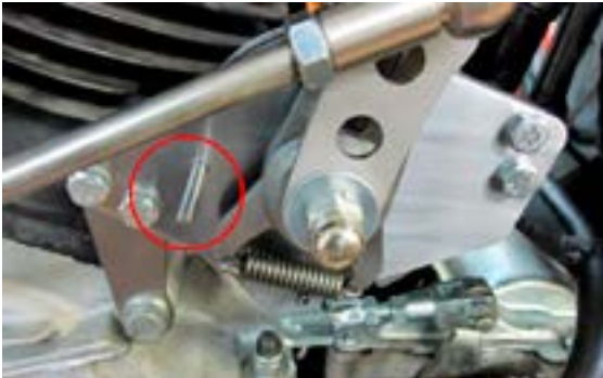
Pin placement - 2nd gear position
