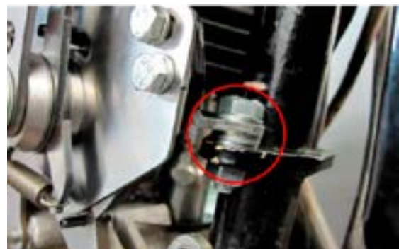
Installation without stock clutch release cable
