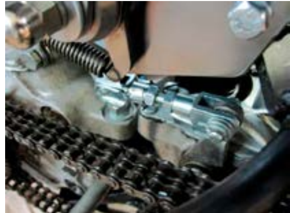
Shifter linkage with clevis
