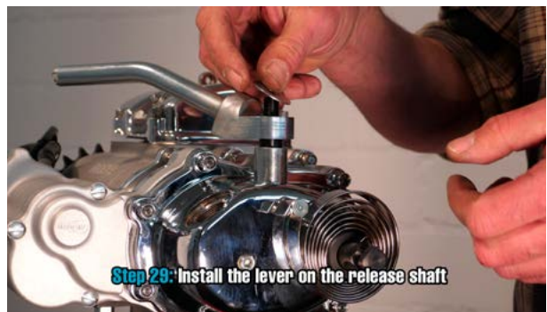
Step 29 Install the lever on the release shaft
