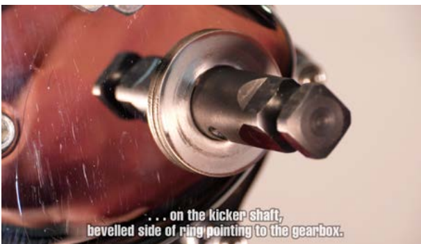
Step 24 Install the BAKER spacer ring on the kicker shaft, bevelled side of ring pointing to the gearbox.
