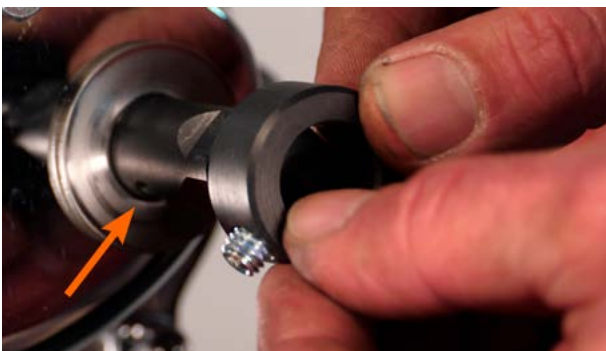
Step 25 Secure the CANNONBALL spring fixator with the locking screw in the hole provided.
