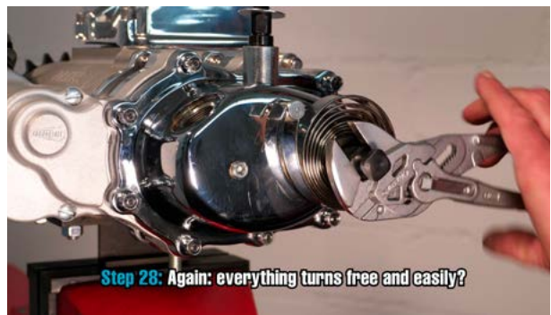
Step 27 Install the kicker spring Step 28 Again: everything turns free and easily?
