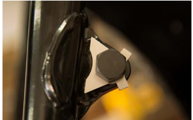
Put brake anchor bolt 8 with tab washer 9 underneath head through mounting bracket on fork tube.
