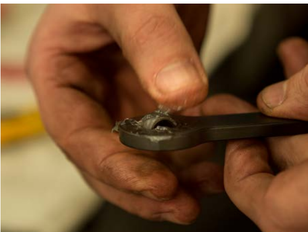
Grease brake anchor pivot bearings 20 from all sides. Turn balls until they are completely covered with grease.
