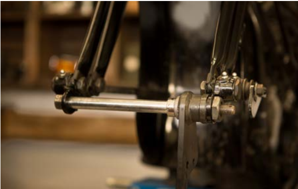
After sleeve nut 22 is tightened turn bracket. It must move freely.
