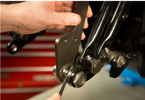
Measure gap with feeler gauge. An endplay of about 0.5mm is what you want.
