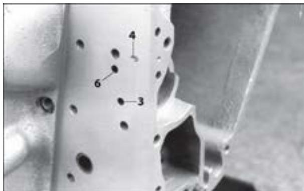
(3) front chain oil, (4) pinion shaft oil, (6) tappet block and cylinder head oil
