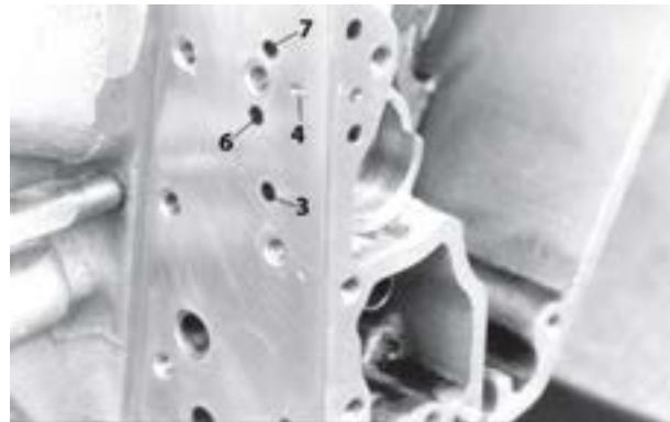
(3) front chain oil, (4) pinion shaft oil, (6) tappet block and cylinder head oil, (7) relief passage
