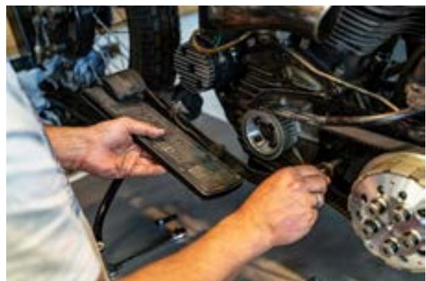
Put the hardened ball into the pressure rod adjustment screw with a little grease, adjust the clutch with some play and tighten the lock nut.
