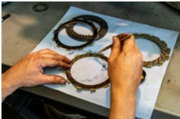
Mount the steel disks so that the 4 ventilation cutouts in the disk are inline of each other and form an air channel.
