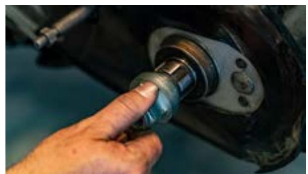
Place the clutch assembly on the transmission input shaft, oil the threads and bearing collar of the nut (large diameter), and lightly tighten the nut.
