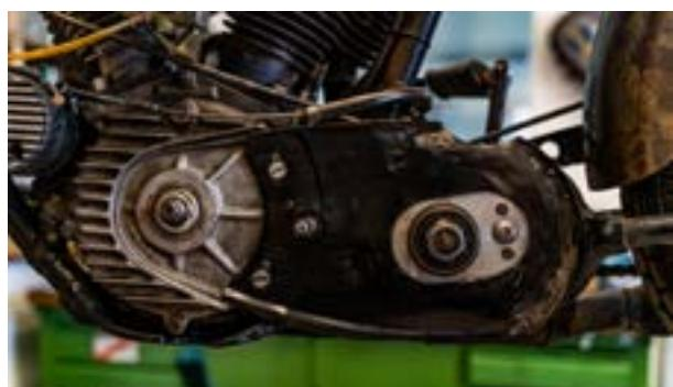
Slightly loosen the gearbox in advance, in order to correctly tension the belt later.
