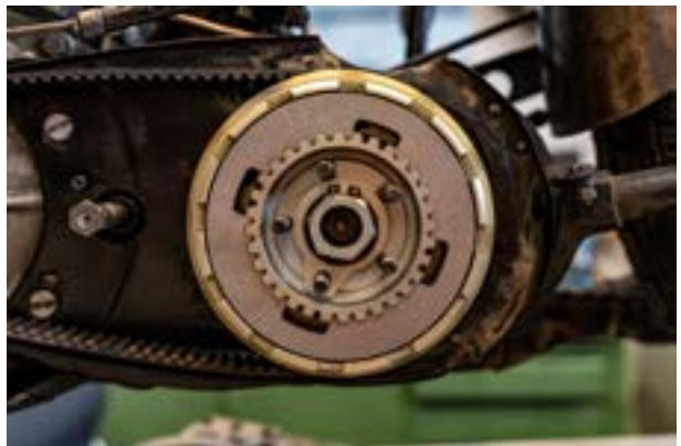
Mount the 5 friction and 5 steel discs alternately.
