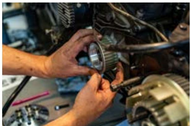
Put the timing belt on and mount the pulley on the adapter along with the determined number of spacers. Tighten the 4 hex socket screws only lightly for the time being, the final tightening with 20 Nm torque and medium-strength threadlocker can be done later with the rear wheel blocked.
