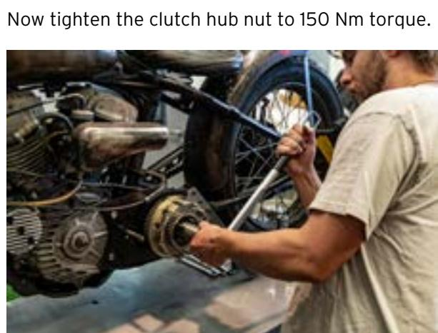
Check that the clutch basket rotates freely and has at least 1mm of circumferential clearance to the inner primary cover.
