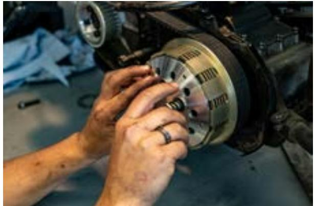
The innermost disc is a friction disc, the outmost a steel disc (see picture).
