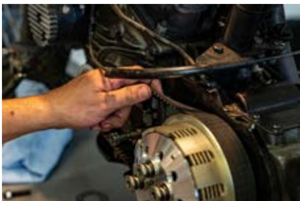
Check the belt tension again after tightening the 3 gear nuts.
