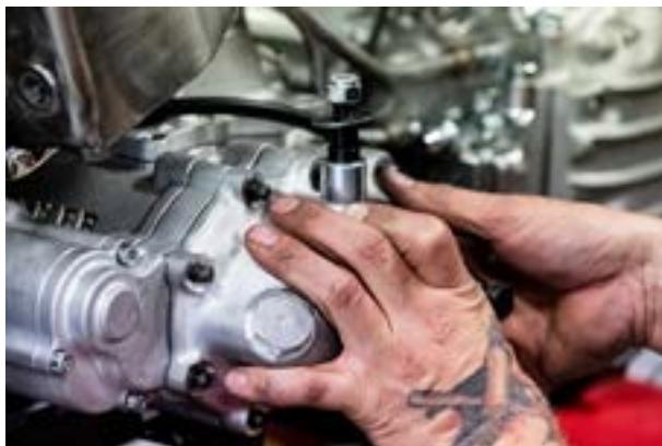
Place first the thrust washer (use existing one) and then the kicker shaft spacer with set screw and slot on the kicker shaft. Tighten the set screw to 9 ft-lbs.
