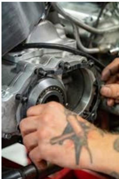
place the locking plate and tighten the nut (50 ft-lbs).
