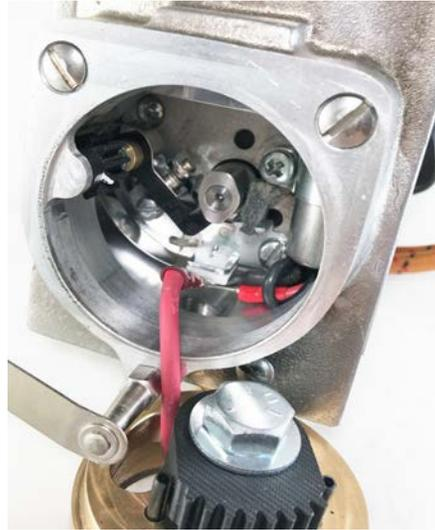
This magneto is designed and built to give you many years of reliable service. Periodically, apply 1 drop of oil to the top of the joint between the bronze timing ring and mating aluminum surface. Operate advance-retard mechanism to spread.
