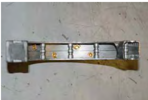
This is how rivets look without the right tool.
