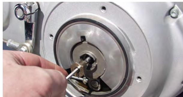
5. Hook the clutch cable into the new Müller segment and mount the latter in the side cover.
