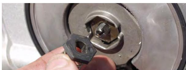
4. Disconnect the cable from the clutch segment, take out segment and put the three balls into the Müller segment.
