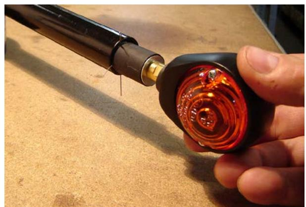
The turn signal unit must be seated so that it can't turn or vibrate loose and the two lenses are parallel with the motorcycle longitudinal axis.
