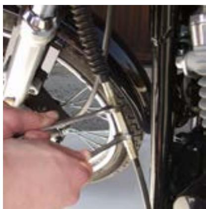
3. Loosen the jam nut from clutch cable adjuster and turn adjuster in to provide slack in cable.
