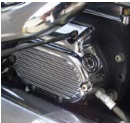
11. Adjust clutch cable with adjuster to provide 1/8" free play at hand lever. Tighten jam nut.
