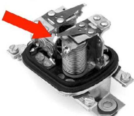
The peak voltage, i.e. the highest voltage the regulator will feed to your battery, is adjusted on 13-541 by bending the hooked tongue of voltage control coil. Again, bending it up and increasing the tension of the spring, will increase the peak voltage and vice versa. (pic. 2, upper arrow) The ACCEL regulators have, again, a coiled spring at the place of a reed spring. Adjustment is accordingly.
