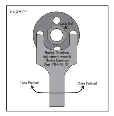
Note: Maximum preload is reached when the locknut and adjusting nut are turned to the end of the threaded eye (no thread showing). This distance is approximately 1/4". Do not turn the locknut past the last thread!
