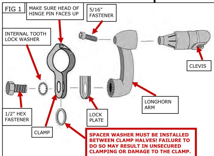
**SPACER WASHER MUST BE INSTALLED BETWEEN CLAMP HALVES! FAILURE TO DO SO MAY RESULT IN UNSECURED CLAMPING OR DAMAGE TO THE CLAMP.**
