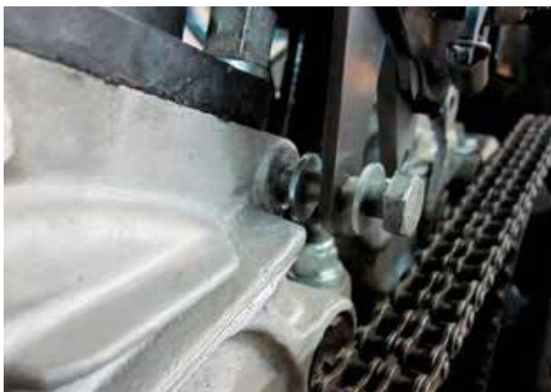
Place washers as required for stressless installation
