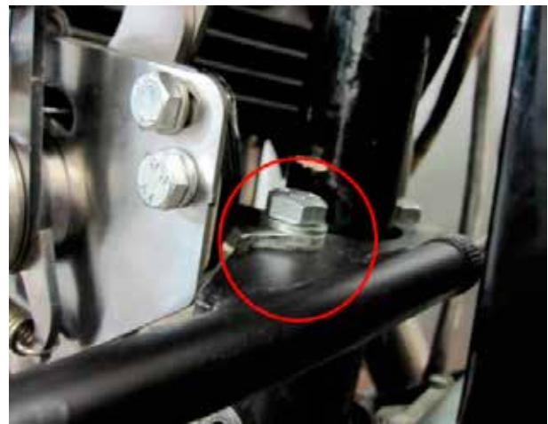
Placement of rear shifter ratchet support angle
