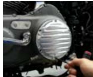
2. Install the backing plate using the provided spacers and bolts. Torque to 90 - 100 in-lbs (10 - 11 Nm).
