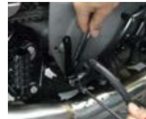
6. Install the new clevis to the master cylinder and mount it to the brake pedal using the supplied hardware. Torque to 17 - 22 ft-lbs (23 - 30 Nm).
