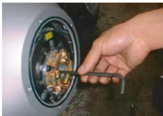
3. Loosen the spring retainer evenly, unscrewing the 6 M6x16 flange head screws a little bit each time using a 10 mm socket wrench. Remove the spring retainer and screws and set them aside.
