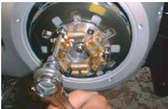
8. Cut out the standard gasket with scissors (if necessary) as shown in the photograph or put the O-ring of the later models instead (WW 57-980).
