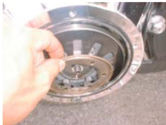
4. Bend the 6 VP base plate tabs to roughly the same angle as the pressure plate center. If bent too far there is no cause for concern.
