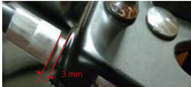
10. Put on the derby cover and tighten the bolts crosswise. A derby cover spacer may be required (WW 80-908). Finally, tighten to a torque of 9.5-12.2 Nm. (84-108 in.lbs) Depress the clutch lever and if the action is smooth then the installation is complete.
