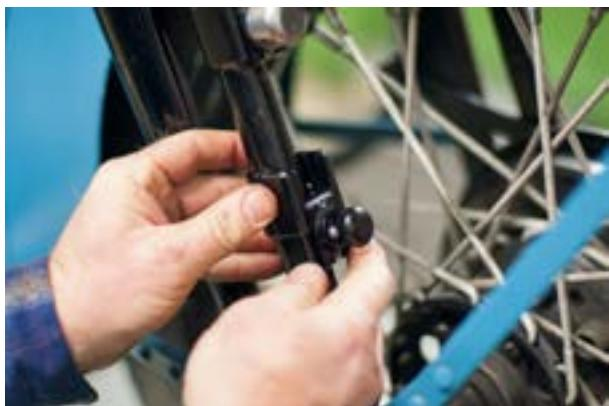
Before installing the clamps on the legs it is therefore recommendable to oil all components and push the sliders through the clamps a couple of times, if necessary with light taps of a rubber mallet, until all parts move without major effort.
